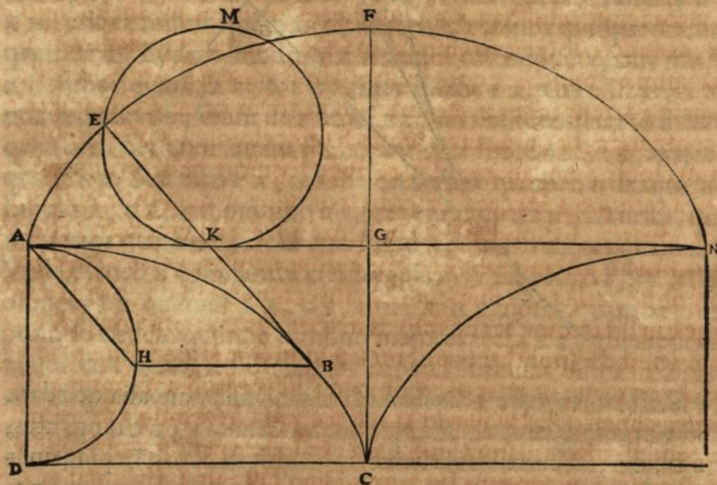
Describatur enim circa A D, axem cycloidis A B C, circulus genitor A H D, cui occurrat B H, basi parallela, in H, & jungatur H A. Quia ergo B K tangit cycloidem in B, constat eam parallelam esse
