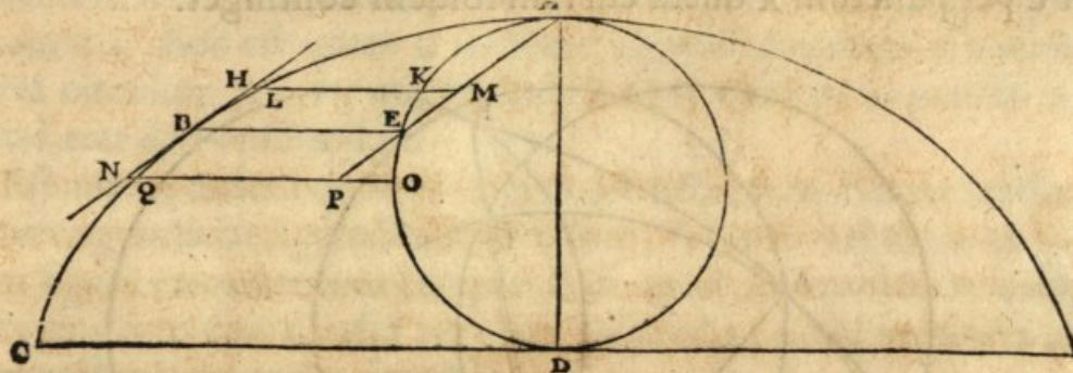
mo versus superiora velut H, & per H ducatur recta basi cycloidis parallela, quæ occurrat cycloidi in L, circulo A E D in K, rectæ A E in M. Quia ergo K L est æqualis arcui K A, recta autem K M minor arcu K E, erit recta M L minor arcu A E, hoc est, rectâ E B, sive M H; unde apparet punctum H esse extra cycloidem.
