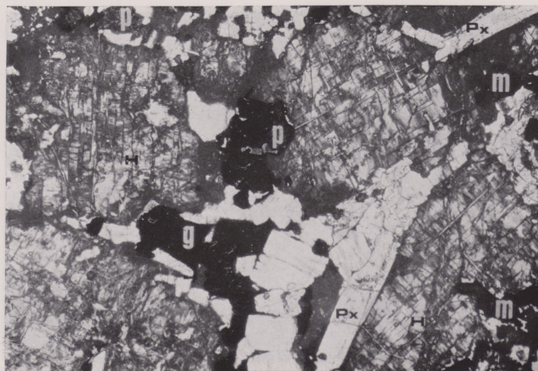
Fig. 2—Textural aspect of the metasomatite: H—hydrogrossular; Px—pyroxene of the salite-ferrosalite type; m—titaniferous magnetite; p—perovskite
