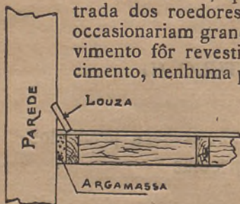
Fig. 34 — FAXA DE LOUZA CONTORNANDO AS PAREDES
